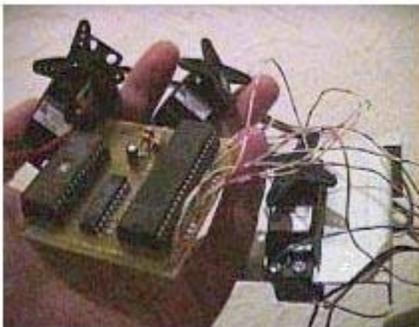
The third robot I brought was my Baby3 robot. It's the least likely to be finished by the contest. So far it's just 3 servos and my 8031PCB. So far the servos go through a test pattern, but I do not have a walking robot yet. My hopes are to make a hexapod walking robots using the electronics shown. Maybe there'll be more to show by the next meeting.
