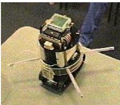
Another nice feature of the ROACH robot was that at the top was a DIP header for attaching a 8051 MCU board. This was used for development purposes and once the logic was figured out, the software was burned onto the 8751 onboard the ROBOT, and the 8051 MCU temporary board was removed.
