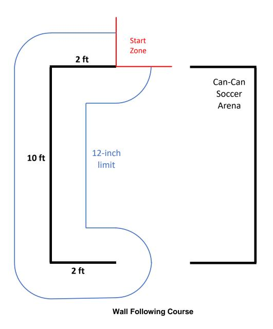
**Course:** The course consists of the walls that make up one side of the Can-Can Soccer competition arena. The course has two 2-foot sections that are set apart by a 10-foot wall section. The 3 walls are connected at ~90 degrees.
