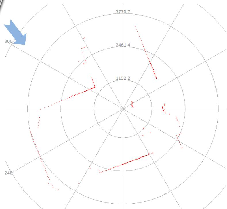
**RPLIDAR system use a low power (<5mW) infrared laser as its light source, and drives it using modulated pulse. The laser emits in a very short time frame which can make sure its safety to human and pet and reach Class I laser safety standard.**
